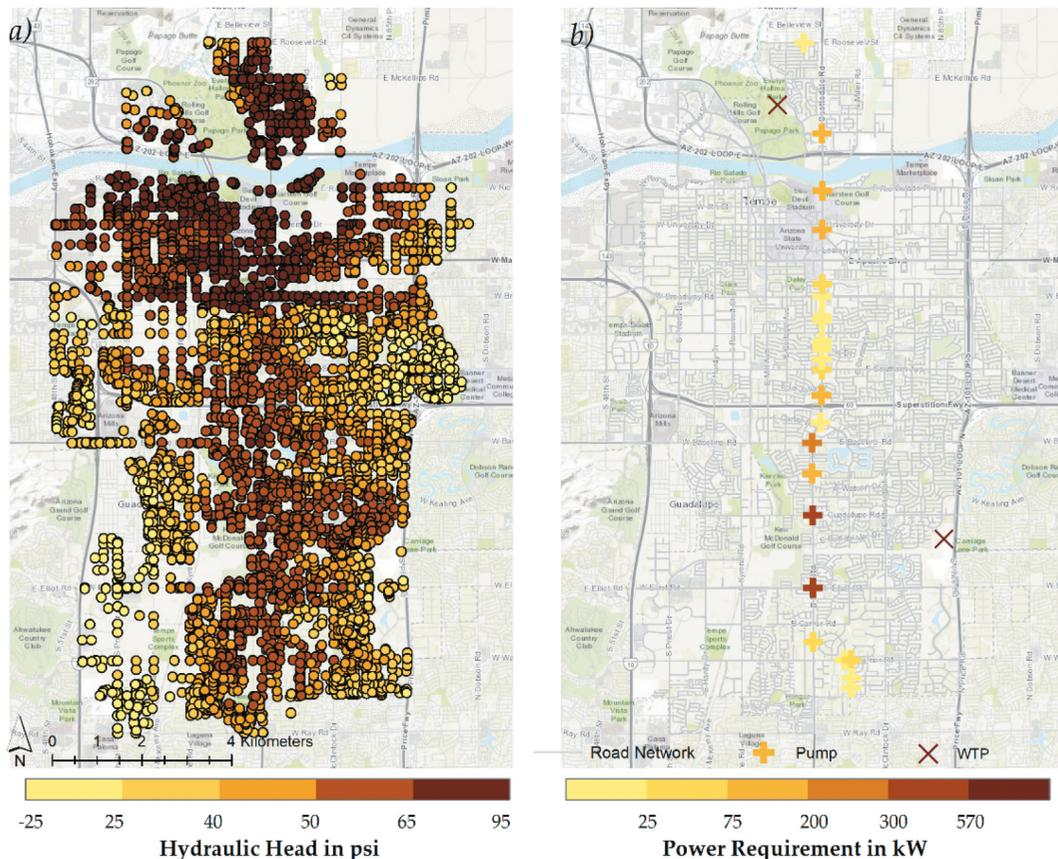
Figure 7. Hydraulic head of each node, pump locations and power requirements of pumps for Tempe, AZ.
