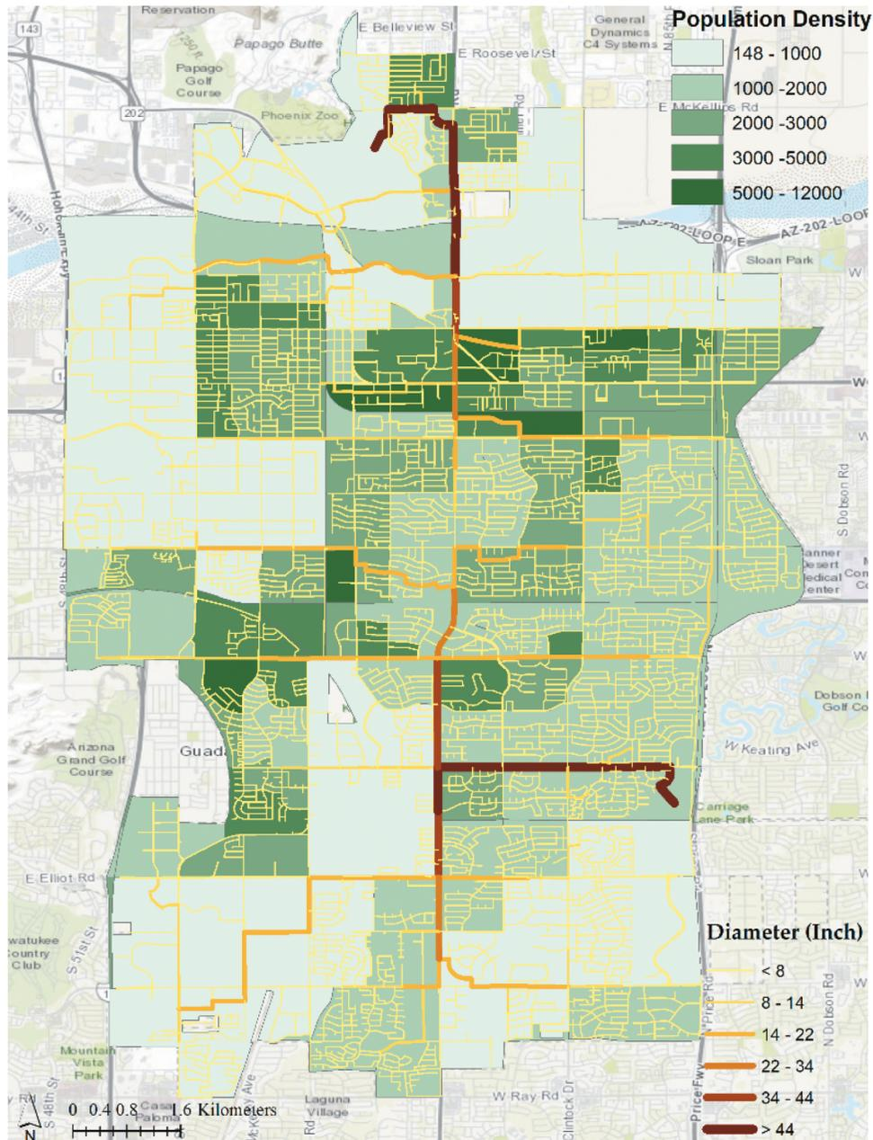
**Figure 6.** Synthetic water distribution network of Tempe, AZ.
