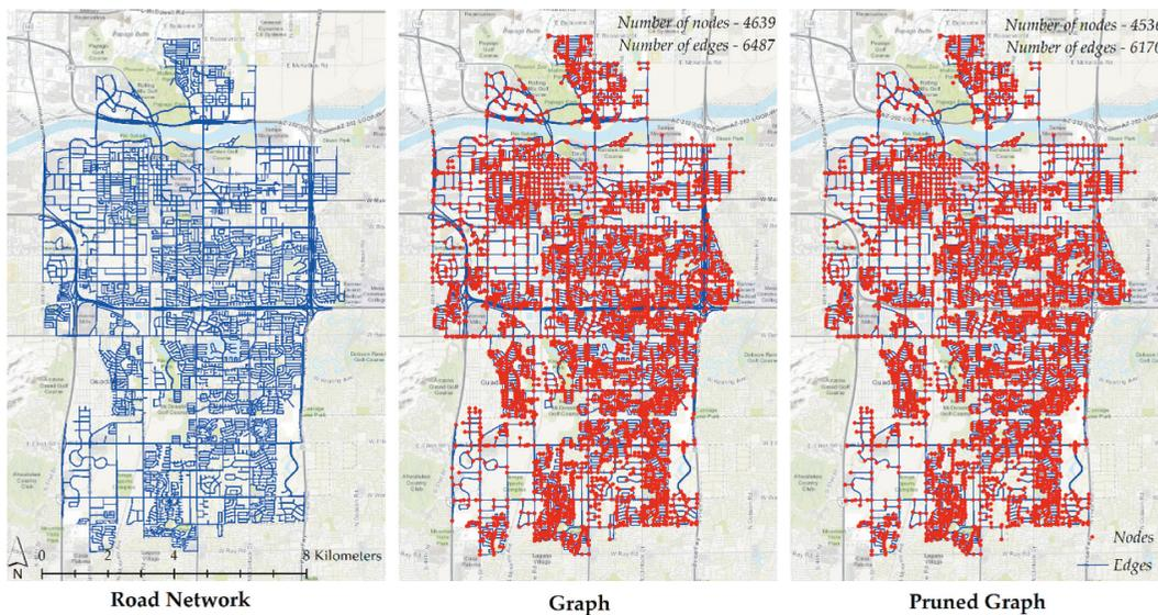
Figure 3. Road network, graph, and pruned graph for Tempe, AZ.
