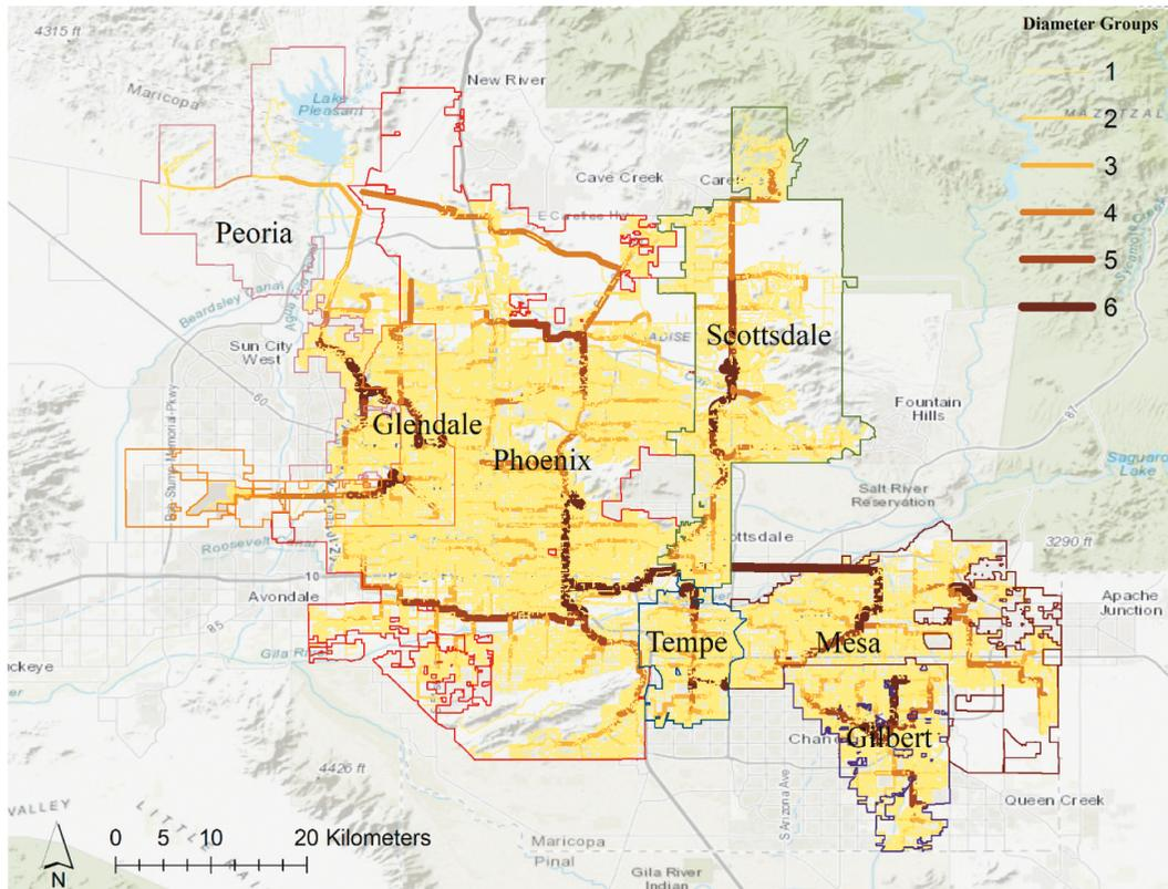
**Figure 8.** Synthetic WDN of Phoenix, Mesa, Tempe, Gilbert, Glendale, Peoria, and Scottsdale (pipe diameters for each city are divided into six diameter groups for visualization).
