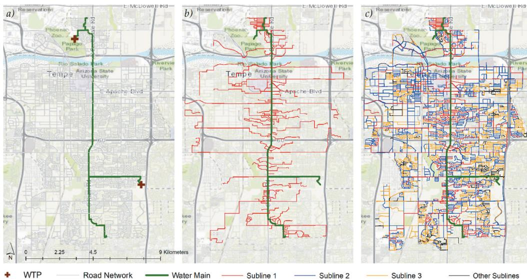
Figure 4. Synthesized water main and other pipes for Tempe, AZ.
