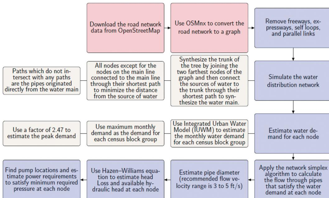
Figure 1. Synthetic water infrastructure generation process.
