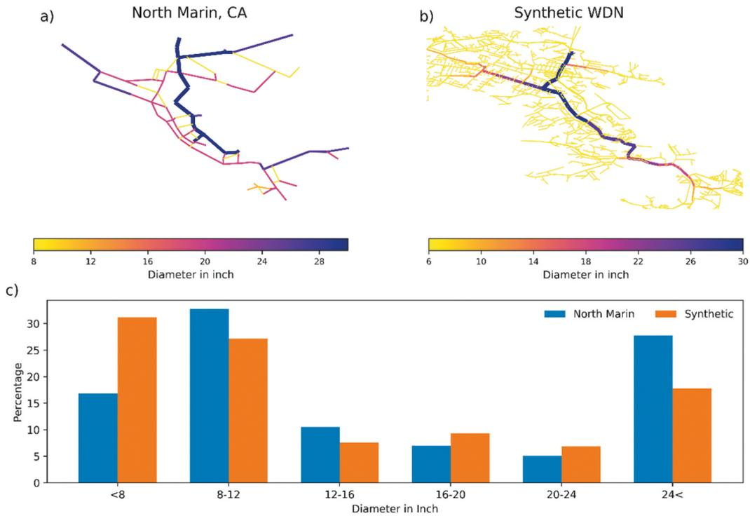
Figure 10. Comparison of the WDN of NMWD and the synthetic WDN.
